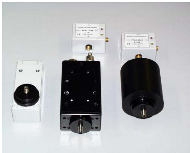
PMH-100 H7422-40 R3809U Detector for the 'Fibre Out' version of the Zeiss LSM-510
