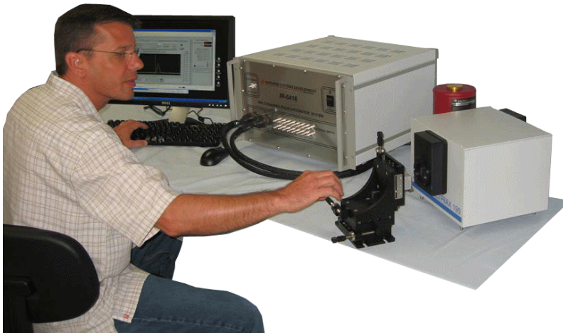
TESTING IR-6416 FEMTOSECOND DATA ACQUISITION SYSTEM WITH SPECTROMETER LASER DIODE, AND X-Y-Z TRANSLATION TABLE
